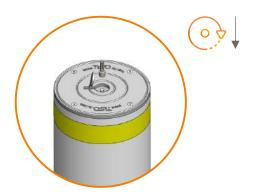
Turn the drill adapter clockwise to lowered the bollard
